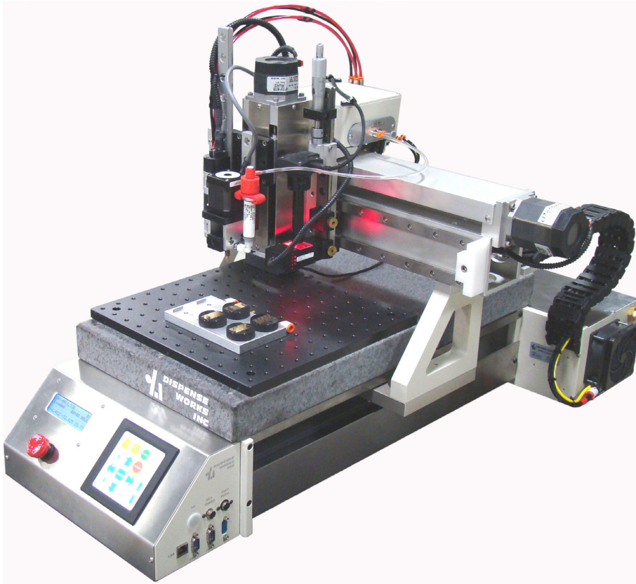
The RPX 1215 Robot features a 2" thick 12" x 24" granite base.
