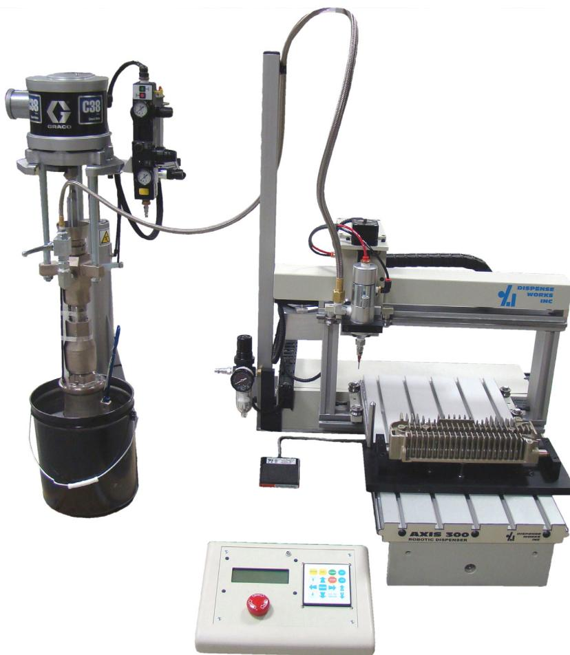
***The Axis 300 Robot is shown with a high pressure spool valve and a 5 gallon pail pump.***
