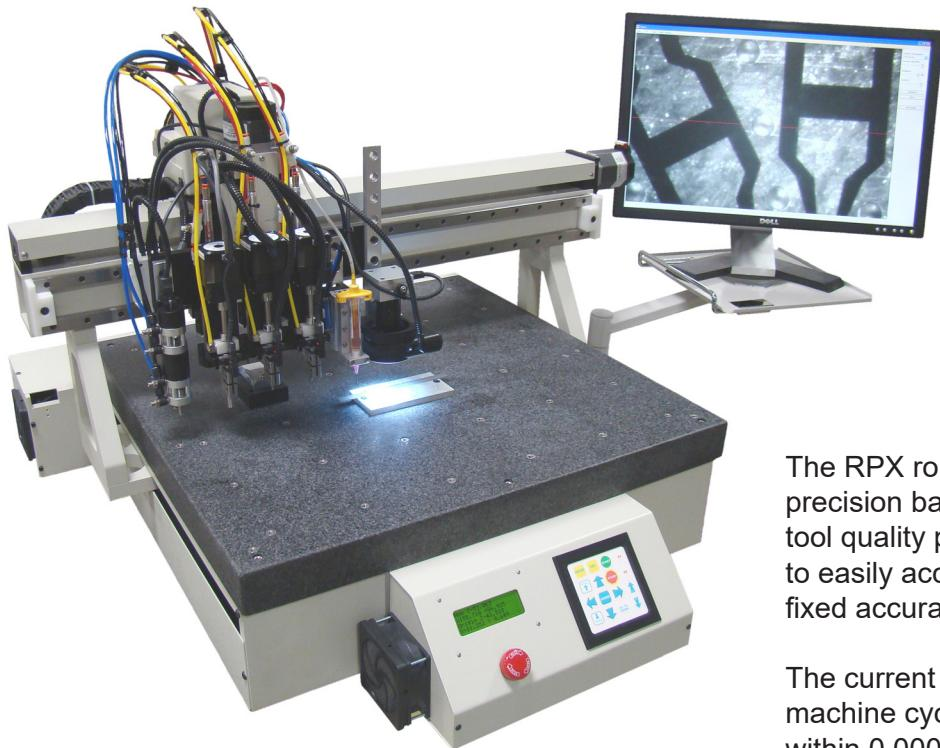
For precision assembly of sub-miniature electronic components using the integrated vision system.
