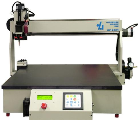
**RP-2424 Robot w/Programmable Auger**
