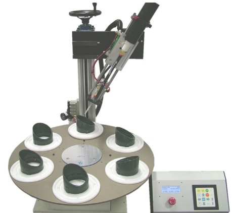
Ring Dex 14 with Rotating Nests Adhesive application inside lamp housings. Removable nests for quick changeover.
