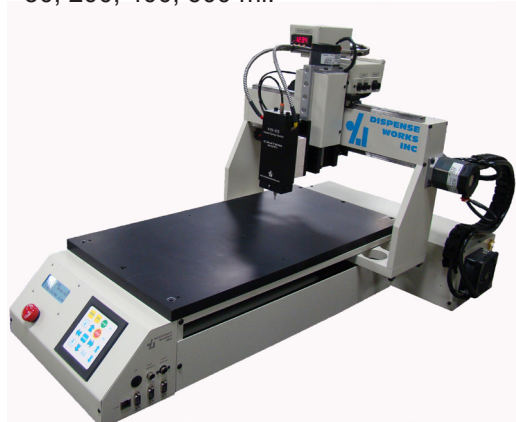
RP 1215 Heated Glass Syringe Mount Heated dispensing head with PID digital temperature control and feedback.
