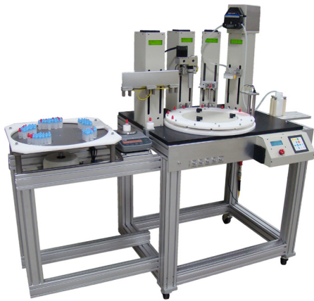
Ring Dex 18 with Base and Accumulator Great low to mid volume production center for filling, capping and tipping. With scale.
